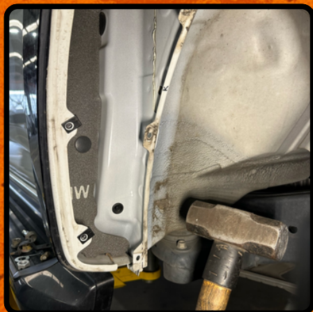
STEP FOUR: Flatten body seam
