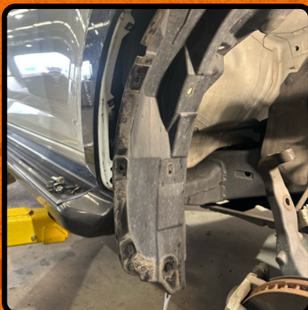
STEP TWO: Peel back the inner guard
