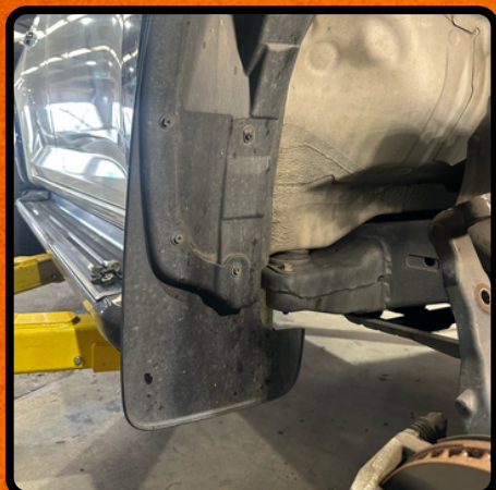
STEP ONE: Remove the Mud Flap
