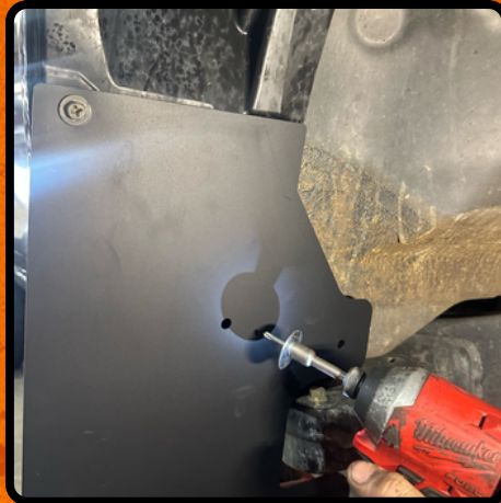
STEP TEN: Install the Mud Flaps. Use the longer screw for the outside hole.
