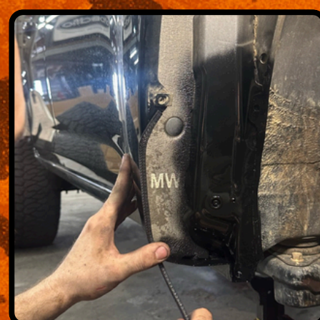
STEP NINE: Apply the provided pinch weld and cut to length
