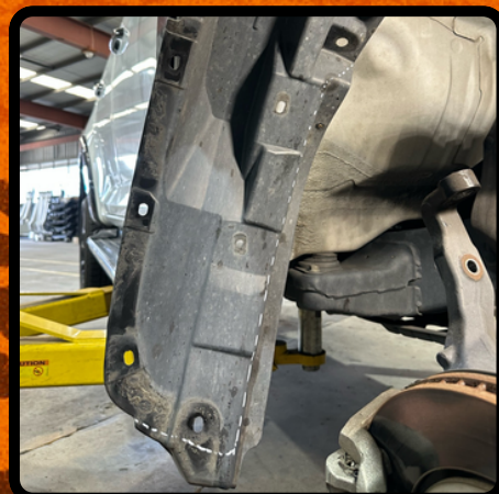
STEP THREE: Mark out the inner guard and cut
