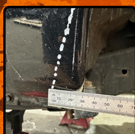
STEP SIX: Mark out guard, 30mm
